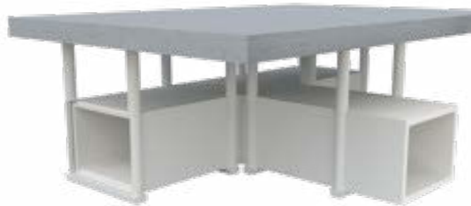
Take-off point on horizontal duct
